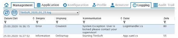
The log files are stored in the **Logging** subfolder. This is located in the same subfolder in which the **TitriSoft.exe** was installed. The tracer files are stored for 6 months.
