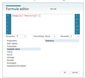
When the method is selected in the work list, the sample variable appears as a numeric input field. Alternatively, a variable created in the Settings Center can be used directly in a calculation, for example of a result variable. In this case the input field also appears automatically in the worklist.
