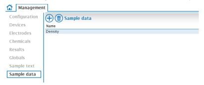
In a calculation, the variable type **Sample** is selected and the corresponding variable is chosen.
