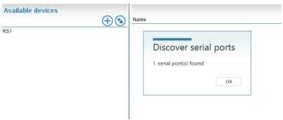
Hereby **RS1** refers to an internal port. In the right part of the window the properties of that internal port are shown and can be set.
